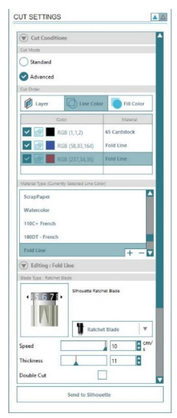
Cut out all piece first using a low pressure setting for the blade on the fold lines so it will not cut completely through the card stock. This will help with the folding and eliminates the use of a folding scoring board.
