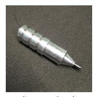
Or you can use an embossing blade at a low pressure setting. Please do not cut these lines with a blade since this weakens the fold.
